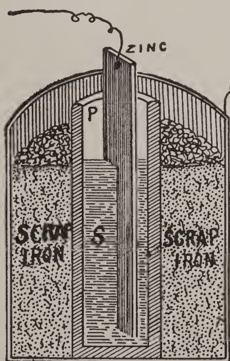
FIG. 67. — A Tomato-Can Cell; Sectional View.
