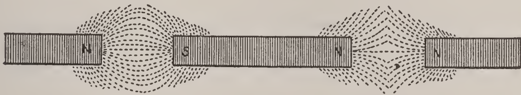
FIG. 15. — Lines of Force between Like and Unlike Poles.
