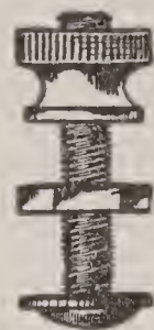
FIG. 94. — Binding-Post removed from the Carbon of a Dry Cell.
